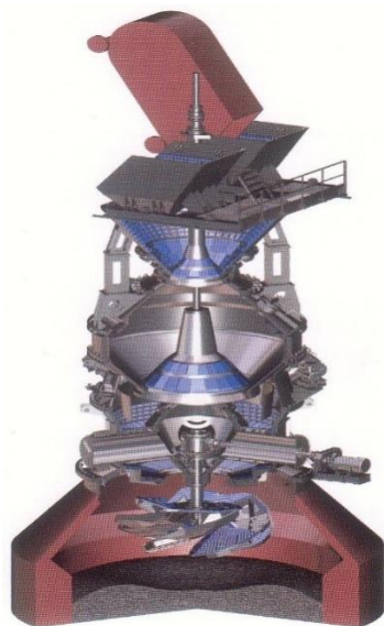
Fig-3 Rotary Charging Unit (RCU)
