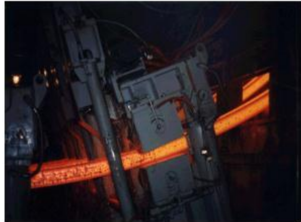
Figure 5 - Straightener Withdrawal Units for Strand Unbending
