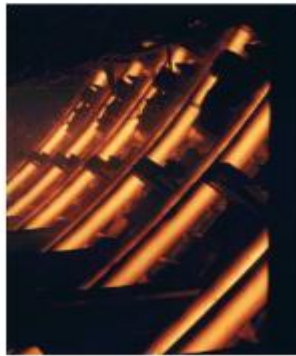
Figure 4 - Curved Section of Multi-Strand Beam Blank Caster prior to Unbending
